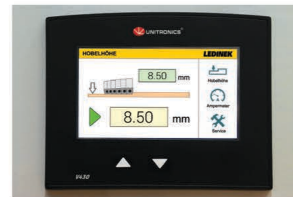
Touchpanel for adjustment of thickness, with current display, overload protection and advanced functions.
