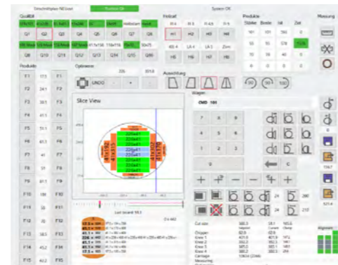
Touchscreen display for band saw control
