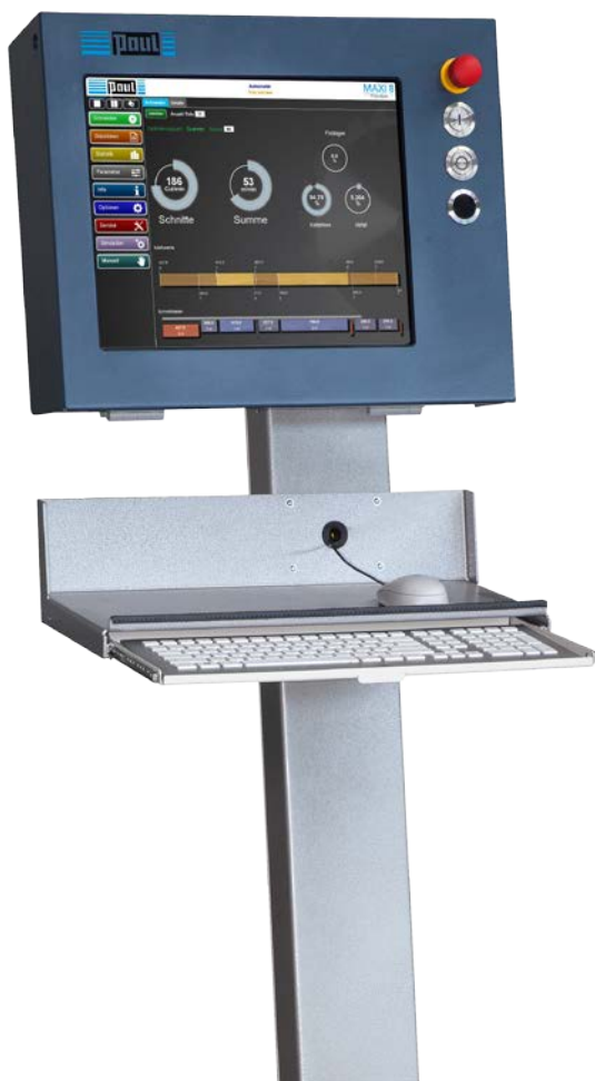
Fig. 5: MAXI control Operator terminal with touch panel, keyboard and mouse
