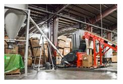
Efficient material discharge via suction system or screw auger
