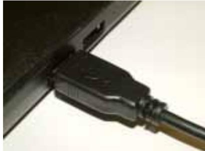
To send your saved logs to the PC, connect the EVO-CHIPS device to your PC using the USB cable that was delivered with your device. Carefully loose the protection cap on your EVO-CHIPS and plug in the USB mini B connector. The bigger connector has to be connected to a USB slot on your PC.
