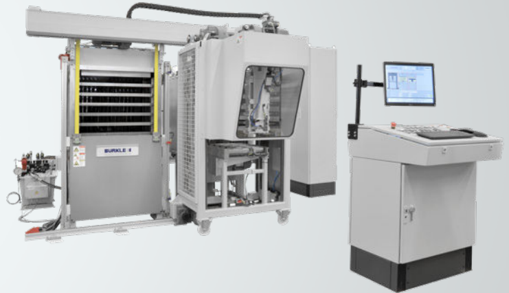
Press line with hot press, cold press and carriage for medium volumes.
