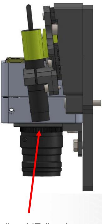
Inclined IR line laser pointing at the mirror
