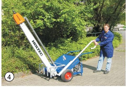
① Cutting assembly with completely stellite armoured guide bar (100-250 cm). Available with **STIHL**-scratcher chain, carbide tipped scratcher chain or chipper chain
