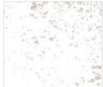
polyalphaolefin (PAO) air release: 12 seconds
