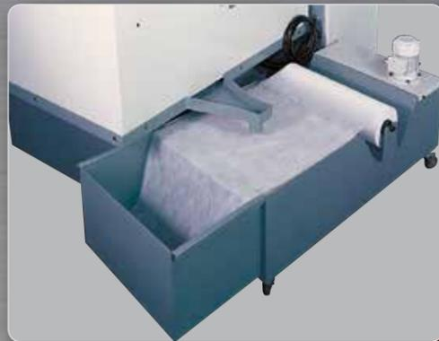
Coolant tank with paper filter
