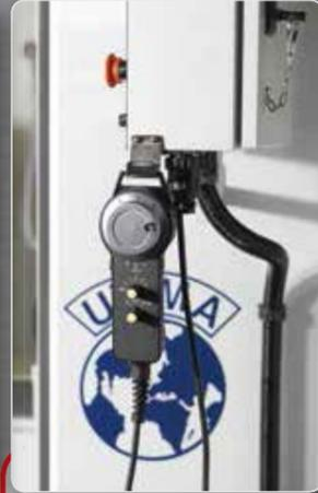
Electronic handwheel to move axis
