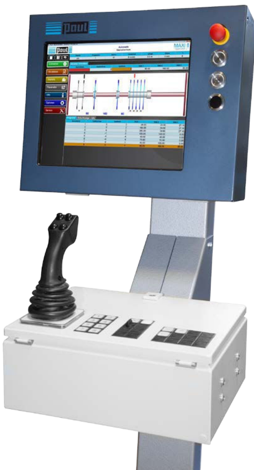
Fig. 13: MAXIRIP control terminal with touch panel and joystick.
