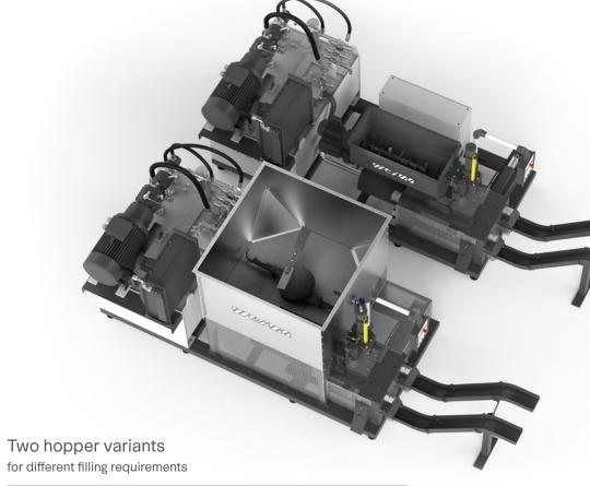
Depending on your needs, you can choose between a large-volume feed hopper for flexible filling by means of a forklift truck or lifting and tipping device, or compact material buffers (chip agitator) for continuous, mostly automated filling, where the material falls directly into the screw conveyor channel. Both hopper systems can be equipped with a practical level gauge that safely switches the machine into standby mode when idle until new loose material is fed in again.
