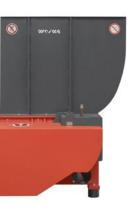
The hopper fulfills several tasks at once. First, the material to be shredded is fed through it – manually, mechanically, or by conveyor belt. The generous opening makes it easy to fill even very large parts. A decisive factor for shredding, however, is its special design, which is rounded at the front and thus effectively prevents material bridging. Even with bulky parts, the shredder cuts itself free. If required, hopper extensions and lids with gas pressure springs are available.
